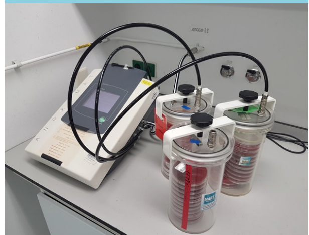
Figure 1. Microaerophilic incubation of H. pylori cultures and the Campylobacter jejuni ATCC 29428 as growth control by the Anoxomat (Mart Microbiology, Drachten, the Netherlands)
